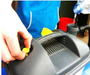
Ensure the generator is not connected to the power whilst filling
